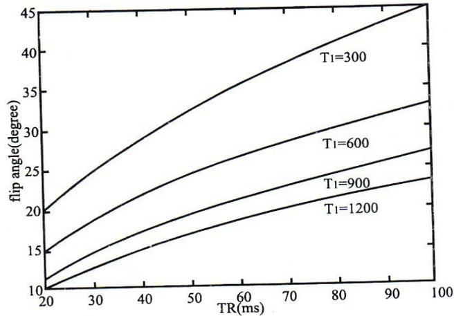
Fig. 1. Graph of optimum flip angle as a function of time of repeat for several  $T_1$
