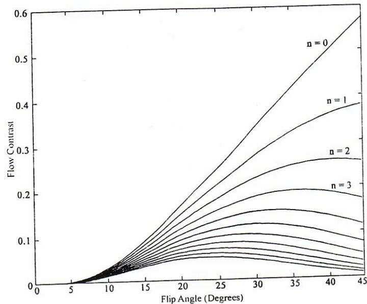
Fig. 2. Graph of low contrast versus flip angle for different n. Parameters ([TR/TE] 40ms/7ms)
